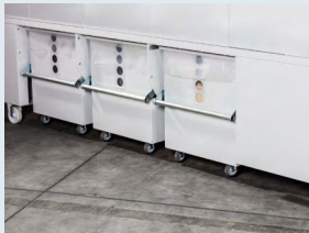
Clamp the chippings container into place
