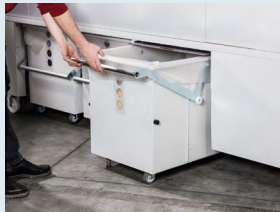
Reinsert the chippings container and remove the dust compartment
