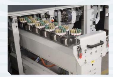
The bottom sanding stations are arranged vertically and therefore easily available for a sanding belt change. The belt lengths of the bottom sanding stations are identical with the belt lengths of the top sanding stations.
