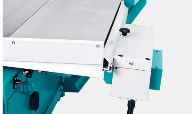
Rip fence pneumatically lowerable | T7074
